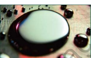
long-term experiments with an aluminum interface. However, liquid metal is safe with polymers, as well as nickel, copper, ceramic, and silicon. When storing liquid metal, it is important to keep it contained and limit its exposure to oxygen so that it does not develop dross. Materials such as silicone or DuPont™ Krytox® can be used to contain it.
